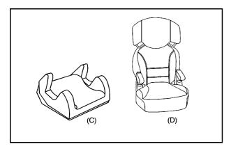
A booster seat (C-D) is a child restraint designed to improve the fit of the vehicle's safety belt system. A booster seat can also help a child to see out the window.
